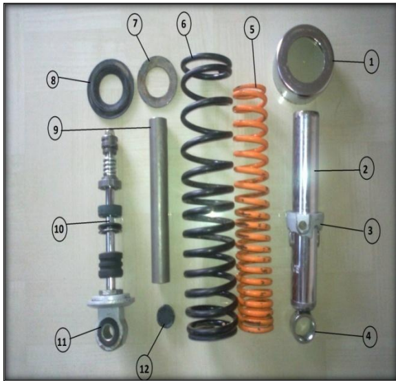
Fig 1. Elements of Twin tube rear shock absorber
